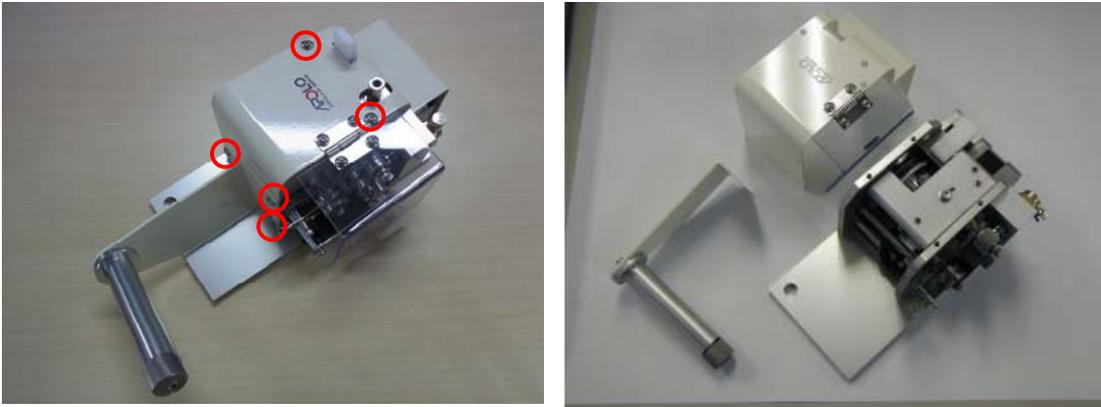
(2) Loosen the set screw "1" for alignment cutting blade shaft and the setting nut "2" to adjust the shaft position. Then move the blade shaft position to match the center of the cutting blade and V groove of the lower roller.
