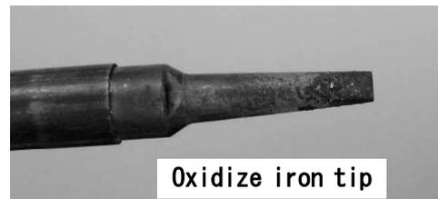
Do NOT file the iron tip because iron plating may be peeled off, then the iron tip cannot be getting wet with solder.
